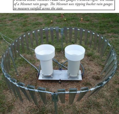
The second rain gauges are identical to the current ones installed. They are a tipping bucket rain gauge. This type of rain gauge has a small bucket that tips and empties whenever a certain amount of rain fills the bucket. The water is collected by a funnel, then it flows into the tipping bucket. The bucket works like a seesaw with a container on each side. A magnetic switch counts the number of tips, which is converted to rainfall accumulation.
