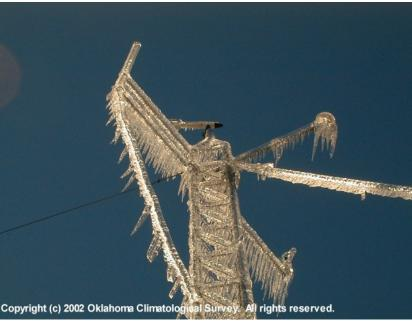
humidity and radar, they can determine if a station is affected by ice accumulation.
