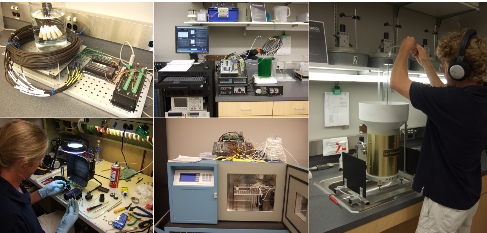
Clockwise from top left: Soil Moisture Calibration, Temperature Calibration Bath - calibrates soil temperature, Rain Gauge Calibration, Air Temperature Moisture Susceptibility, Wind Direction Sensor Rebuild
