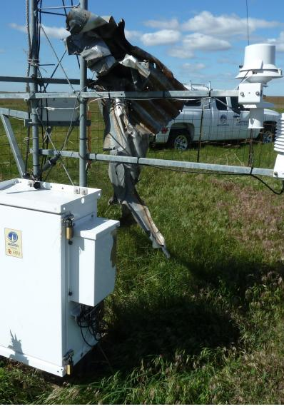
One-minute wind and pressure measurements indicated that the tornado passed the El Reno Mesonet tower around 4:21 p.m. The winds peaked at their highest level, 151 mph, and the pressured dropped to its lowest level, 929.1 millibars, at this time.
